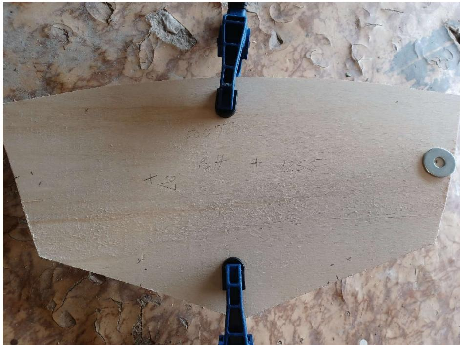
I used the standard 3mm ply for the bulkheads. If you wish to obtain a stronger joint between the kayak sections, you can use stronger ply for the critical bulkheads. I wouldn't use anything thicker than 6mm though. Once reinforced in fiberglass or any other mesh, even the 3mm one will take the load pretty well.
