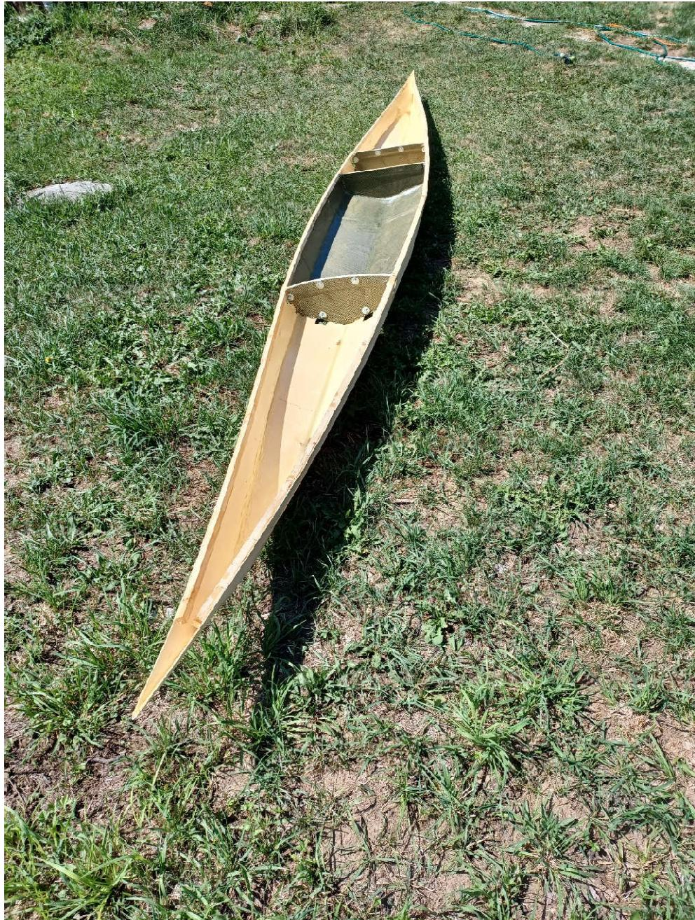
*Do not laminate the external faces of the bulkheads yet.* You will do it after installing the decks, in order to also have the edges of the decks covered with the mesh.
