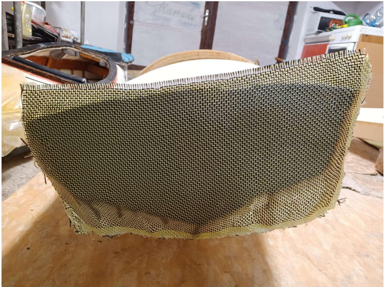
Just follow the manual from now on, as the operations needed for the 3 parts Shrike are done. You can keep the sections apart when laminating the exterior and this will enable you to laminate all the sides in one go (the sections can stand vertically on the ground). However, put them back together when painting a continuous pattern on the hull.
