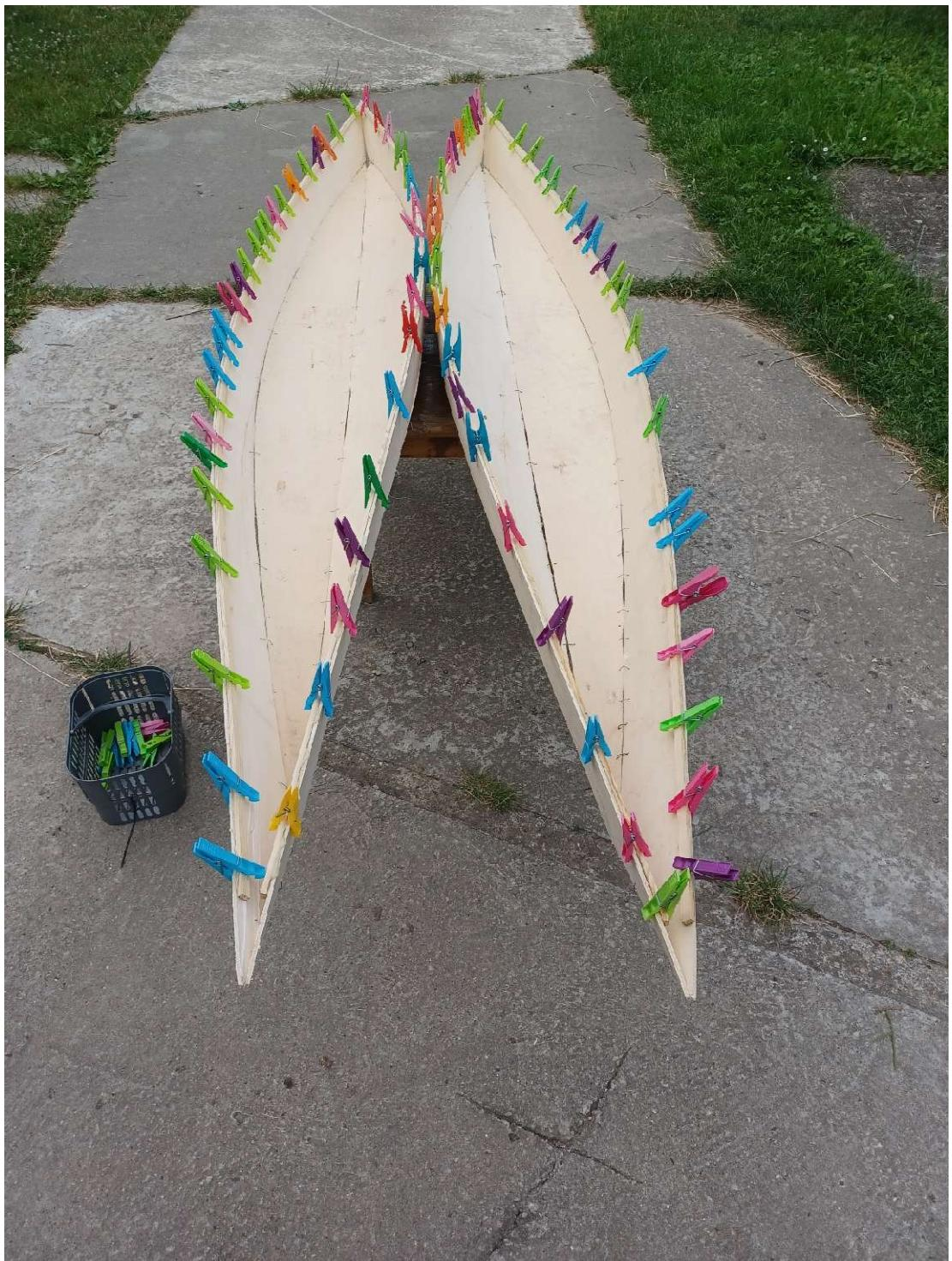
10. Cut and insert the back rest at the indicated position – exactly 142cm from the bow. This position is fixed (it preserves the center of gravity of the boat) therefore the back rest can be epoxy glued to the hull. The back rest length should result 43 cm long. This length can vary only a little if you want to adjust the beam of the boat, but beware of a too sharp taper of the sides (reclining the sides to much)
