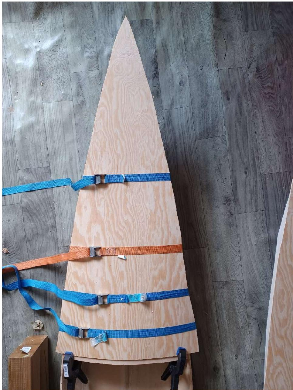
21. Cut a similar piece for the rear deck. It may happen not to have a piece of ply of enough length to cover the rear. No trouble. Cut the deck as long as possible and cover the remaining gap with a new, shorter piece
